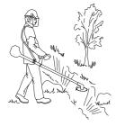
Take great care when cutting a tree that is under tension. A tree that is under tension may spring back to its normal position before or after being cut. If you position yourself incorrectly or make the cut in the wrong place the tree may hit you or the machine and cause you to lose control. Both situations can cause serious personal injury.
